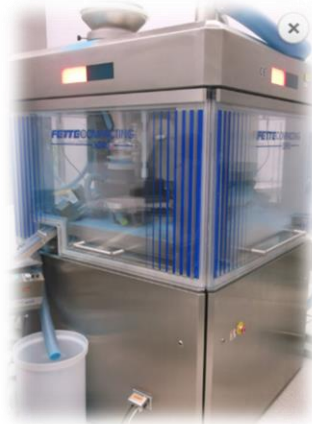
High speed tableting with multi-tip toolings
